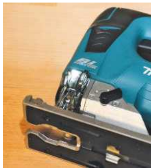
▲ The worklight LED illuminates to indicate the saw is ready for use
